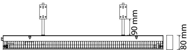
Model showing 2 bearing arms incl. light tube and louvre. Armature housing in aluminium.
